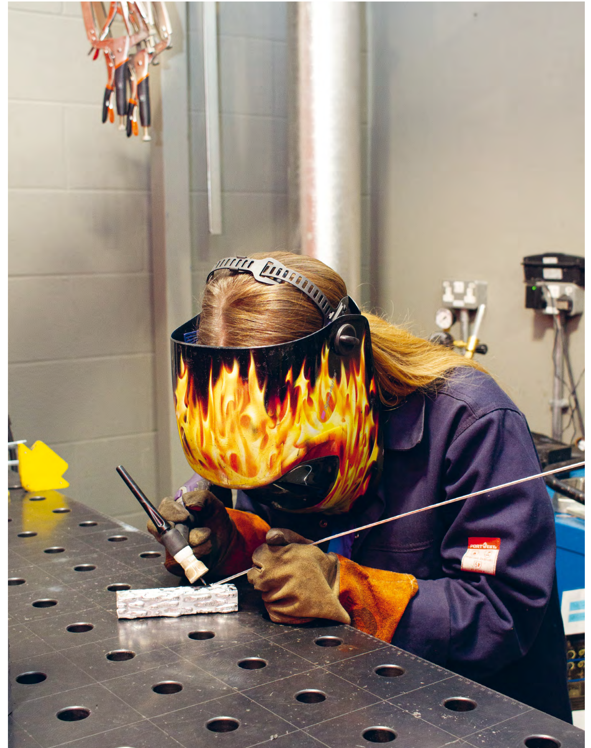
Above: I'm welding aluminum; Next page: First welding lines of club members. It is TIG (tungsten inert gas) welding, which is more difficult to learn than MIG (metal inert gas) welding. The club members learned both types.
